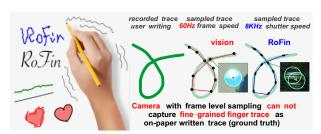
Figure 1: RoFin with shutter level sampling can better record jitters of hand trace compared with frame level sampling.
