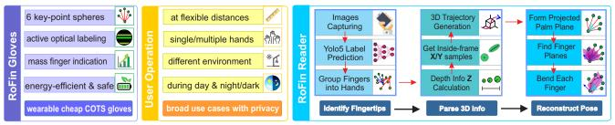
Figure 5: RoFin system overview: composition, workflow and three main tasks.
