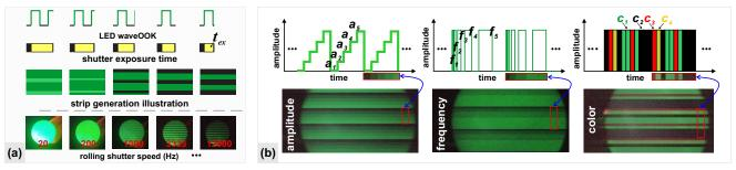
Figure 6: (a) Captured strips impacted by shutter speed. (b) Light feature selection for temporal rolling patterns.
