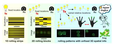
Figure 4: Strip effect from single to multiple light sources.
