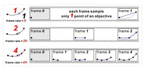
Figure 3: Frame rate vs. tracking granularity.
