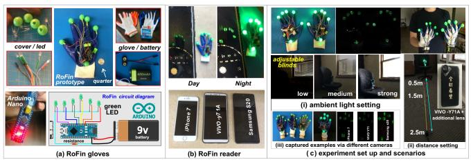
Figure 13: System implementation: RoFin gloves (prototype & circuit diagram), RoFin reader (commercial cameras) and experiment scenarios (varied ambient light strength and distances from 0.5m to 2.5m).
