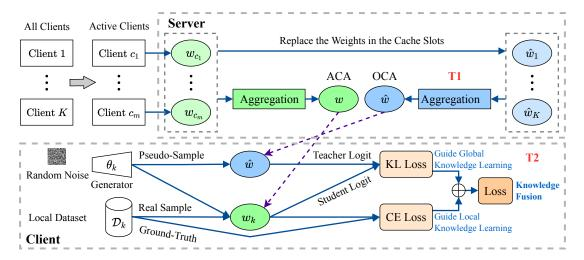
Fig. 1. FedKF Overview. Two key techniques (i.e., T1 and T2) are developed in FedKF. In T1, we develop an active-inactive model aggregation technique to generate an OCA model that represents the global knowledge precisely. In T2, we develop the global-local knowledge fusion technique to enable the local model to learn both the global knowledge (embedded in the teacher model, i.e., the OCA model) and the local knowledge (embedded in the local dataset).
